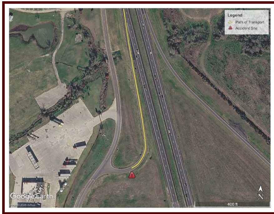
Aerial imagery showing the vehicle accident location at the sharpening curve of the exit ramp.
